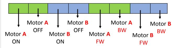
**Example Question:** Enter the values into the register to move the robot forwards and backwards
